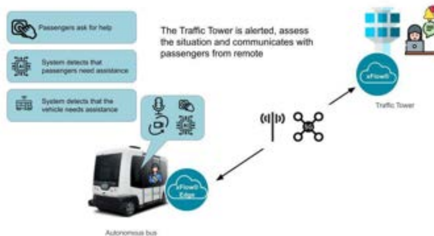
Fig. 2. Use case diagram for a passenger assistance system in autonomous operation.
